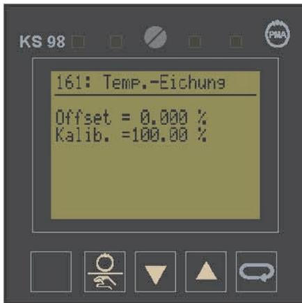
Operation of the KS 98 is particularly simple, whereby only three front-panel keys are needed to configure the sample-specific parameters for temperature, time, and sequence. A practically unlimited number of stages for temperature and time (resolution 1 second) can be stored. The number of stored programs is only limited by the memory capacity, but that is probably large enough for all requirements.
