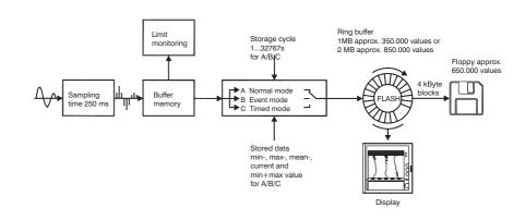
The Engineering Tool (see Accessories) provides the function "Storage period", with which the recording period is computed for the selected configuration.
